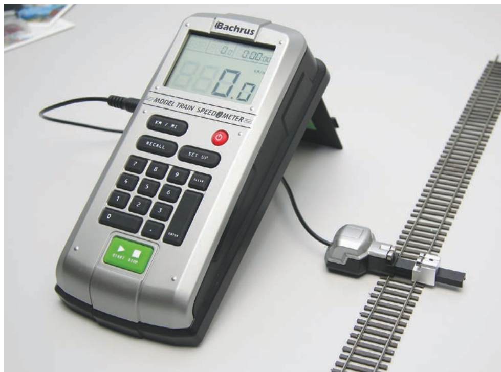
Rolling stand accessory reads the rotation of bearings and translates into a scale speedometer speed display.
